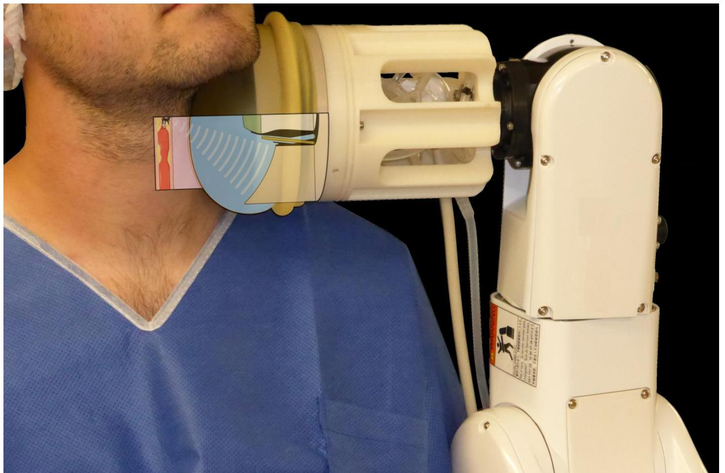
Ultrasound thrombolysis device developed for in vivo thrombolysis tests.
